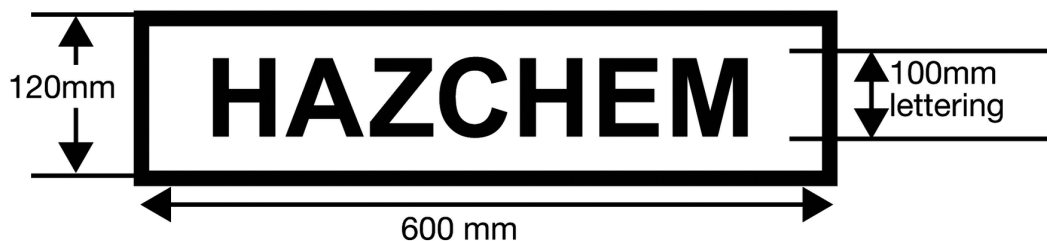
Figure 13.1 Form and dimensions of outer warning placard
