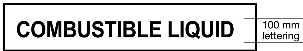
Figure 13.5 Placard for flammable liquid category 4
